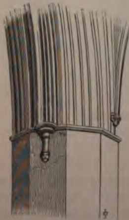
Impost of Piers, Nave, St. Patrick's.
